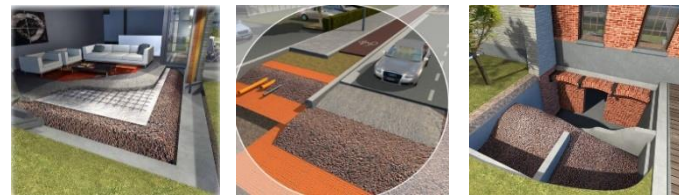
Figure 2: Examples of lightweight expanded clay aggregate in lightweight filling applications
